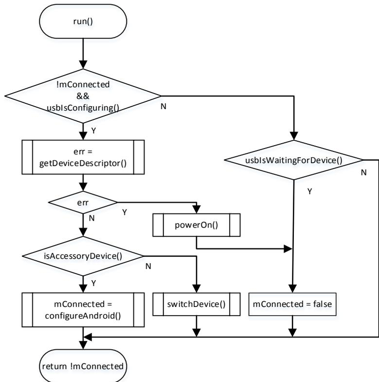
Figure 3: The flowchart of AndroidAccessory::run().
