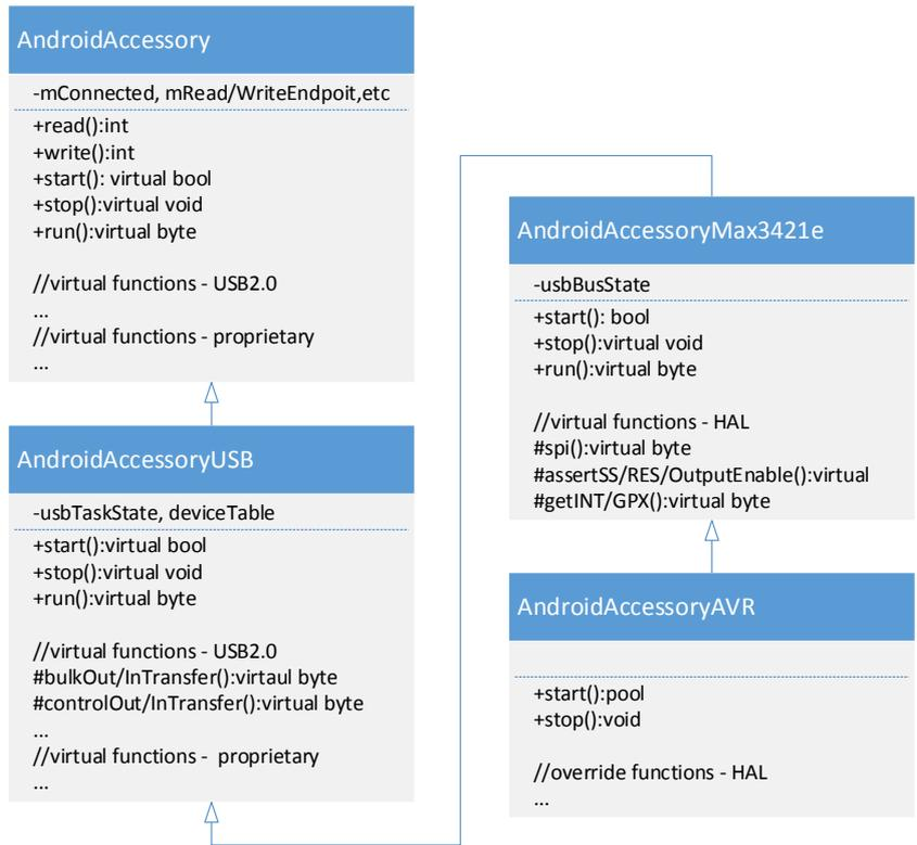
Figure 2: Class diagram of the Android accessory.
