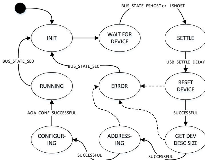
Figure 4: The state machine diagram of AndroidAccessoryUSB::run().
